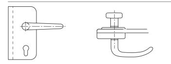
FSB front door furniture with dead knob for use on glass doors feature modified bearings and spindle lengths (door thickness). Door knob is turnable.
