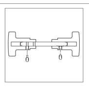
Turnable knob handles are made and supplied by FSB as female sections. Knobsets are created by joining two female parts together using the FSB Stabil-spindle 0102.
