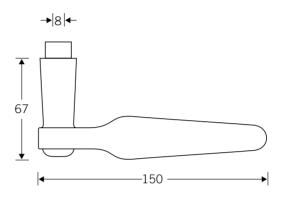
The FSB 1103 lever handle by Hans Hollein is shaped to the hand in classical FSB fashion. Hans Hollein incorporated two specific principles into this model: Firstly, he wanted to keep the user's hand well clear of the edge of the door. Hence the offset between the point of pivot and the grip. Secondly, he wanted to offer a choice of either upward or downward lever position, thus lending the door a flexible identity.
