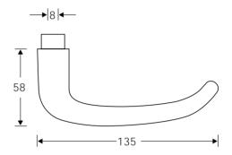
When the UIm Design College was being built in the Fifties, the Swiss architect, sculptor and designer Max Bill with Ernst Moeckel designed a lever handle based on the railway carriage handle common in Switzerland. It entered design history as the 'Ulm handle'.
